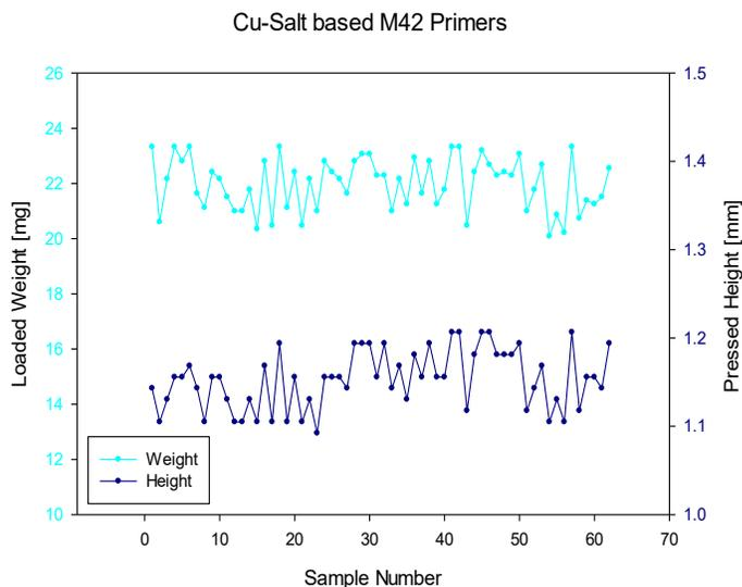
**Figure 7.** Charge weight and pressing height data for Cu-Salt based M42 primers.
