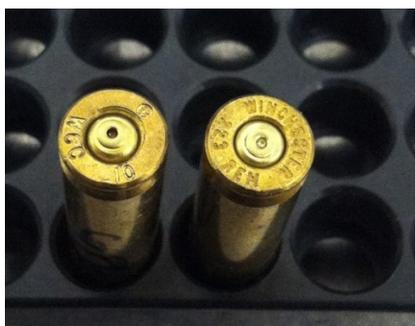
**Figure 9.** Photograph of flow-backed primer cup bottoms from Neyer D-optimal sensitivity testing of K-salt based M42 primers.
