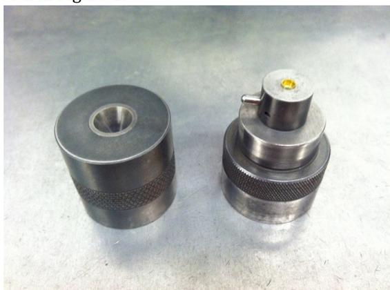
**Figure 1.** Dry loading setup for M42 primers.
