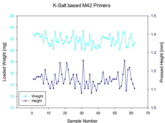
**Figure 6.** Charge weight and pressing height data for K-salt based M42 primers.
