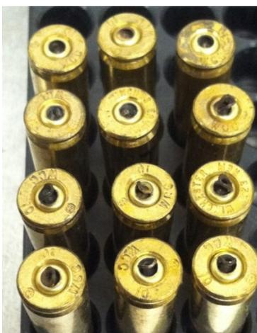
**Figure 8.** Photograph of perforated and punched-out primer cups from Neyer D-optimal sensitivity testing of K-salt based M42 primers.
