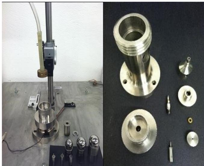
**Figure 3.** Photograph of the ball drop device (left) and the pressure cell device (right).
