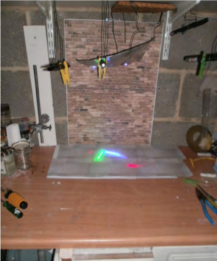
**Figure 4.** This photograph of a laboratory demonstration employs a mirror of the same general type as in Figures 2 and 3 but shaped for and attached at its South end to a West-facing wall as if in latitude  $52^{\circ}\text{N}$ . From the wall, the mirror curves outwards towards the viewer. Four laser pens are suspended around the mirror representing the directions of light from the sun falling upon the mirror at the following approximate times and dates; from right to left:-
